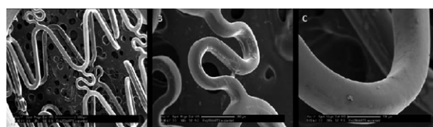
Fig. 9 In situ PEG400diIPTS-coated stent expansion. Low magnification image ( \times 34 ) (A); stent sites subjected to the maximal stress during expansion (B, C). Stents were immersed into buffer phosphate solution for 1 min and then expanded from the initial diameter of 1.8 mm to a final diameter of 3 mm.
